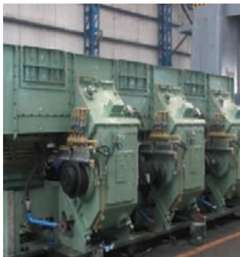
6 Stand Wire Rod Block for Kobe Steel, Japan
