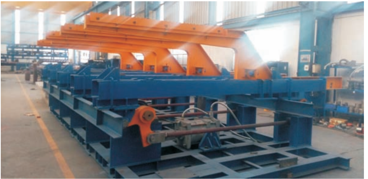
Layer Transfer Arrangement
