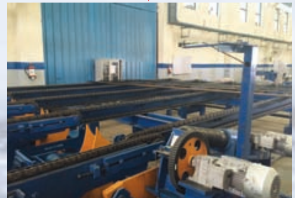
Bar Counter & Separator
